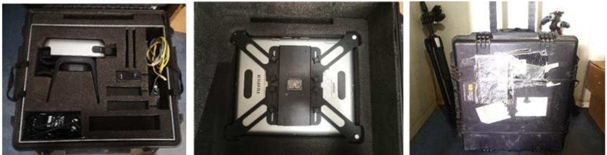
Figure 11. The packaging of (a) the generator and accessories, (b) the detector, and (c) the carrying case (external). *Images courtesy of CIDRZ.*
