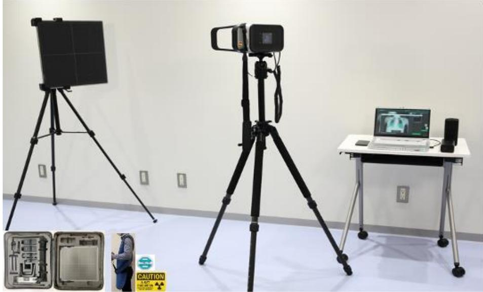
Fujifilm FDR Xair is an ultra-portable X-ray system with ultra-lightweight **X-ray generator (FDR Xair XD2000)**, **wireless FDR X-ray detector (FDR D-EVO II)**, and **HP Console Advance (DR-ID 300CL)** with embedded **application software (DX-CL, Virtual Grid and Dynamic Visualization II)** for image processing. The software also has image editing features to optimize CXR images.
